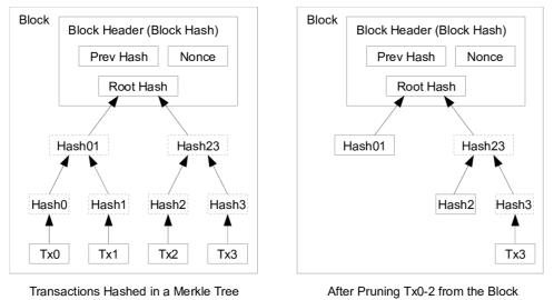
A block header with no transactions would be about 80 bytes. If we suppose blocks are generated every 10 minutes, 80 bytes \* 6 \* 24 \* 365 = 4.2MB per year. With computer systems typically selling with 2GB of RAM as of 2008, and Moore's Law predicting current growth of 1.2GB per year, storage should not be a problem even if the block headers must be kept in memory.
